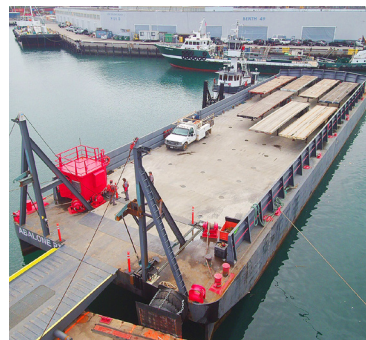
Abalone Pt.: Deck Barge: 2000LT 185'x50'
